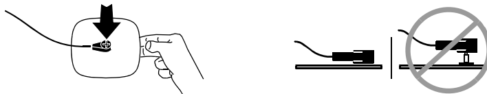
Figure 5-4 Connecting FAST-PATCH Electrodes to Defibrillation Cable
