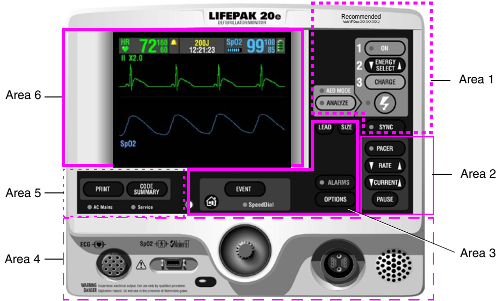
Figure 2-3 Front View without Door
