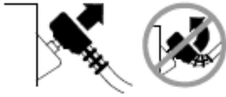
Figure 5-7 Disconnecting Defibrillation Cable from Test Post
